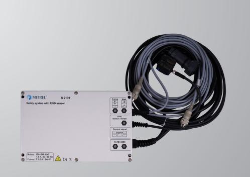
This safety module is designed for test places where protective cover or safety door is used. The module is intended for protection with an RFID sensor and emergency switch. The RFID switch indicates the state (opened/closed) of the door of the cage or cabinet. If the door is opened the safety module will disconnect the measuring circuits from the mains, which results in the maximal protection for the operator. The safety module is equipped also with the emergency
